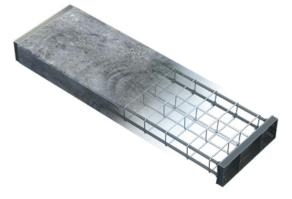
· Side shutters are clamped into position, and the element is poured.
